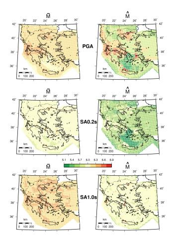
**Fig. 1.** Mean (column 1) and Modal (column 2) magnitudes as a function of PGA; SA(0.2 s) and SA(1.0 s).
