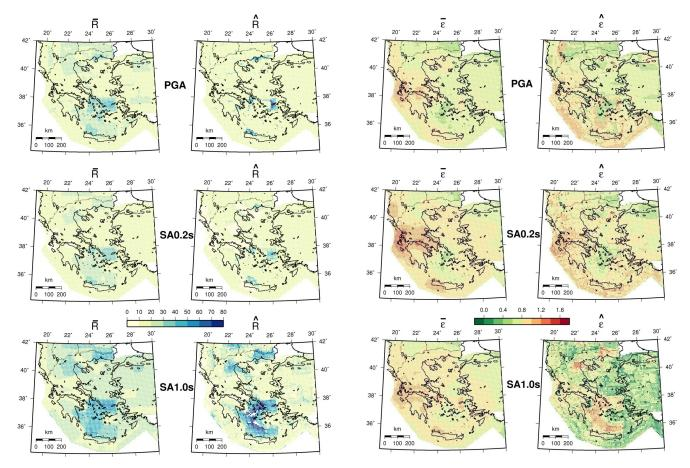
Fig. 2. Mean (column 1) and Modal (column 2) distances as a function of PGA;  $SA(0.2\,s)$  and  $SA(1.0\,s)$ .
