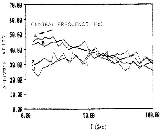
Fig. 2. Seismic spectrum in the time domain for different frequency bands. Note the similar slope of the decay of the curves, implying a linear dependence on frequency of  $Q$ .
