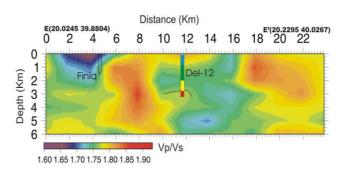
Fig.8. Vp/Vs results versus depth along EE'.
