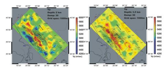
Fig.9. Comparison of PST results with known structure at (a) 2Km and (b) 3.5Km.
