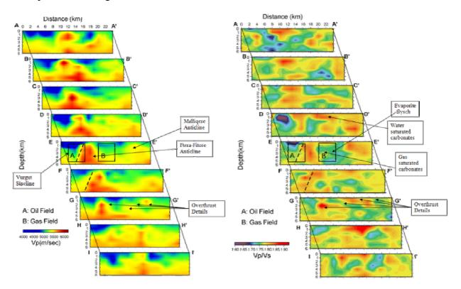
Fig.5. Vertical sections of (a)  $V_p$  and (b)  $V_s$
