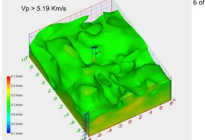
Fig. 10. 3D view of Delvina anticline structure and the surrounding structures based on Passive Seismic results (V<sub>p</sub>>5.19). The production wells are on top of the anticline structure.
