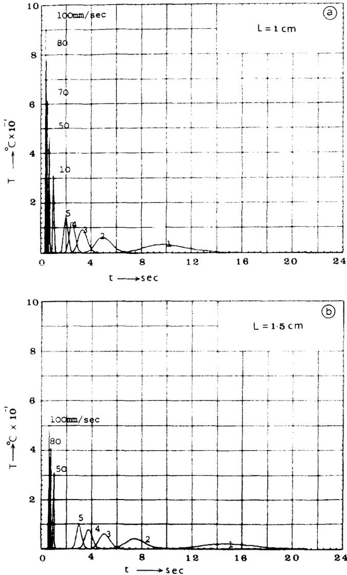
Fig. 3. Temperature at point A as a function of time and water velocity for: (a)  $L = 1 \text{ cm}$ ; and (b)  $L = 1.5 \text{ cm}$ .
