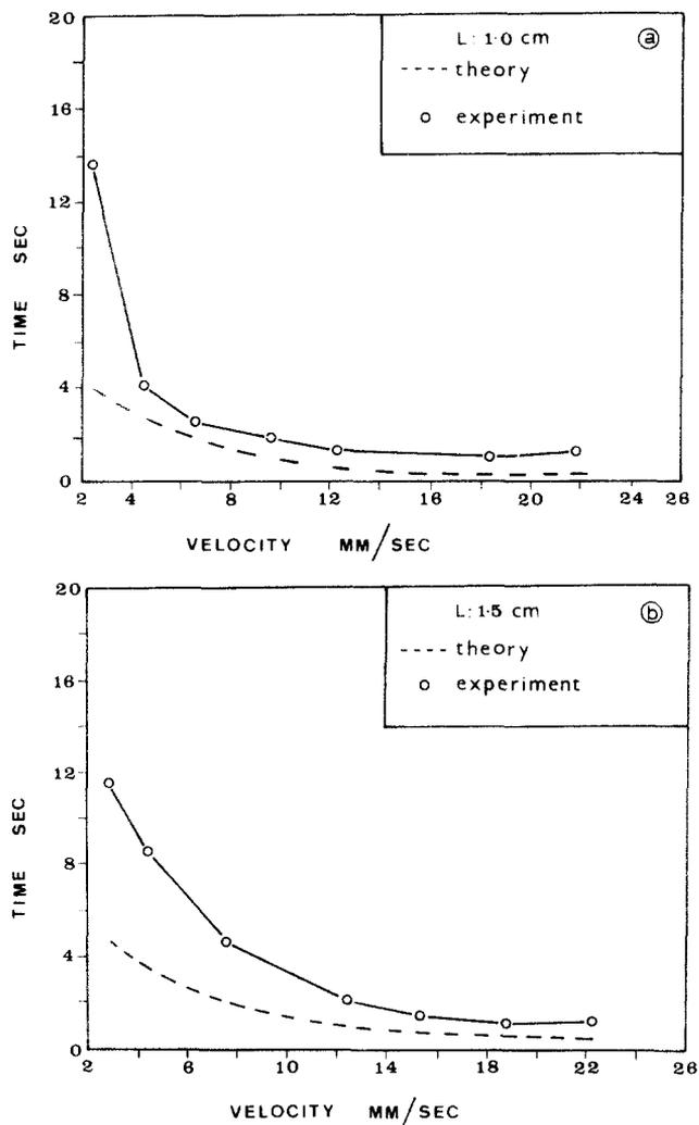
Fig. 5. Comparison between theoretical and experimental results of a 0.25 mm Pt wire for: (a)  $L = 1$  cm; and (b)  $L = 1.5$  cm.
