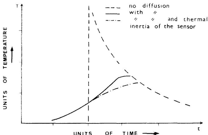
Fig. 1. Typical responses of a temperature sensor with conditions of different diffusion and sensor thermal inertia.
