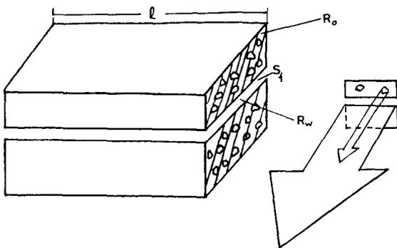
Fig. 1. Double porosity system used to describe the fissured aquifer.
