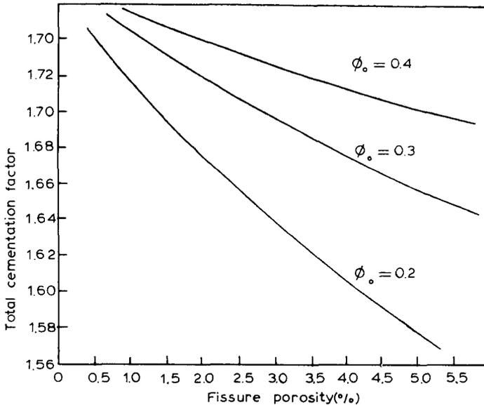
Fig. 4. Equivalent cementation factor versus fissure porosity.
