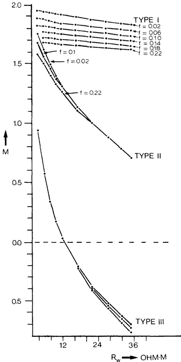
Fig. 3. Equivalent cementation factor versus water resistivity for various degrees of fissuring and for three types of lithology.
