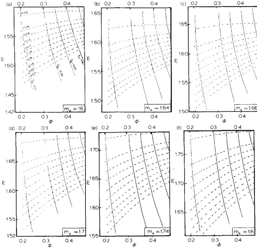
Fig. 2. Relation between the formation parameters of the double porosity model.
