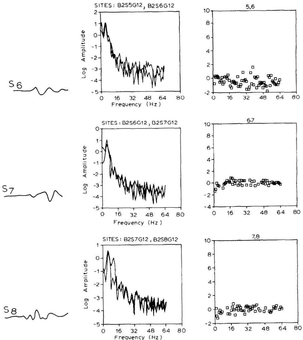
Fig. 4. Wavelets with amplitude spectra and corresponding scatter graphs.
