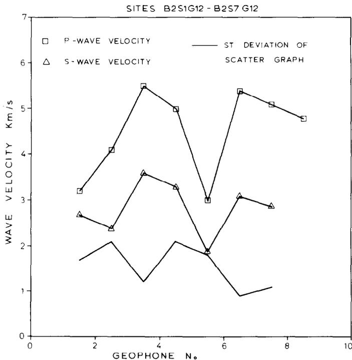
Fig. 5. Variation of P-wave velocity, S-wave velocity and standard deviation of the scatter graphs along site 2.
