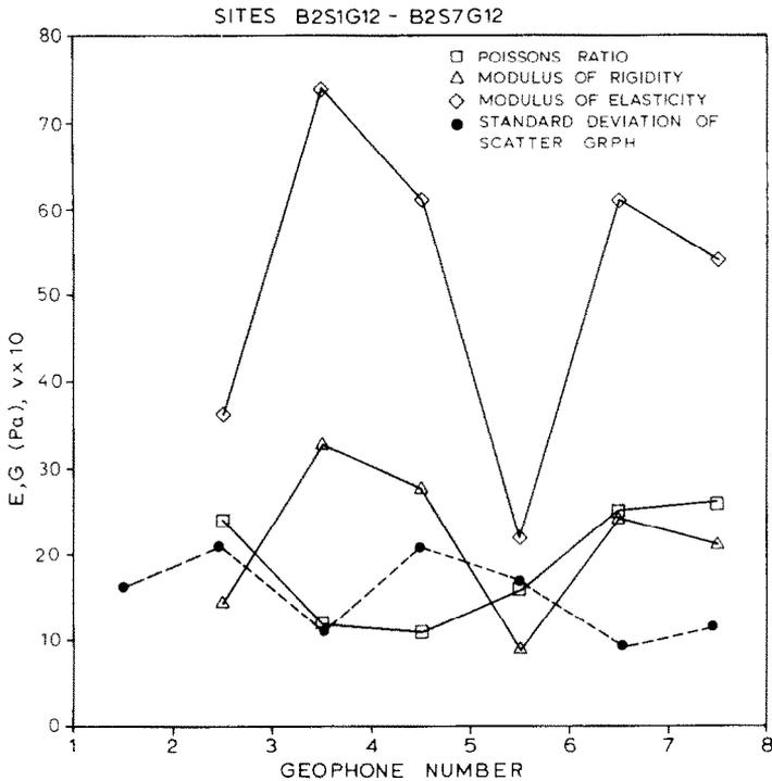
Fig. 7. Comparison of the variation of the dynamic elastic moduli and the standard deviation of the scatter graphs.
