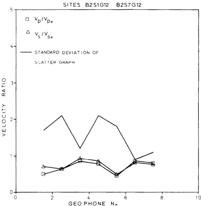
Fig. 6. Variation of  $V_p/V_{p0}$  and  $V_s/V_{s0}$  and standard deviation of scatter graphs along site 2, where  $V_{p0}$  and  $V_{s0}$  are the solid matrix P-wave and S-wave velocities, respectively.
