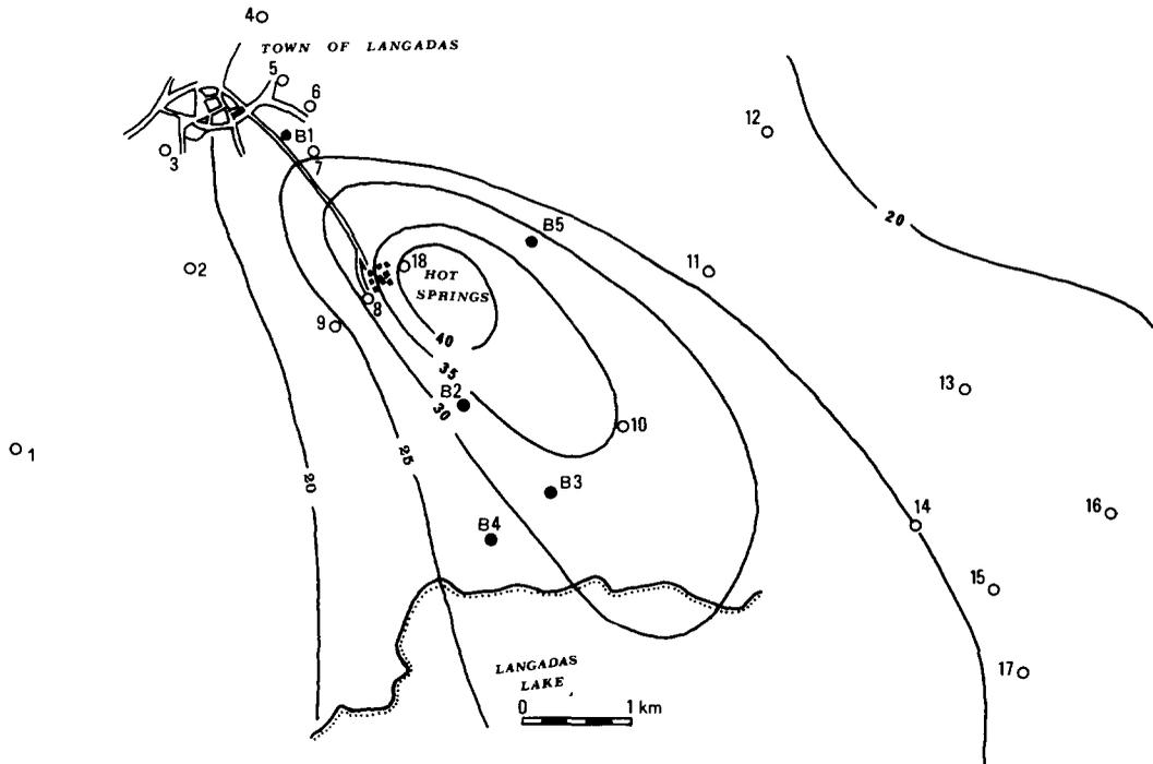
Fig. 2. Temperature contours ( $^{\circ}\text{C}$ ) at 250 m depth over the investigated area and location of boreholes (B1–5 exploration wells, 1–18 water wells).
