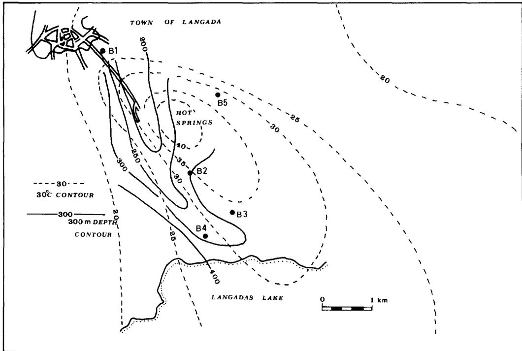
Fig. 7. Comparison between the top of the bedrock and temperatures.
