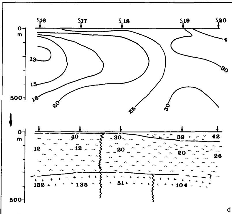
Fig. 5(a-d). Geoelectric models and apparent resistivity for the four measured traverses. (Values in ohm m.)
