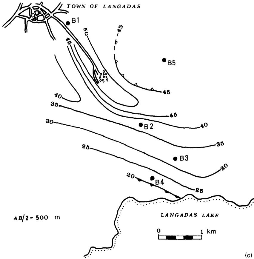
Fig. 6(a-c). Apparent resistivity contours for  $AB/2 = 100, 250$  and  $500$  m.
