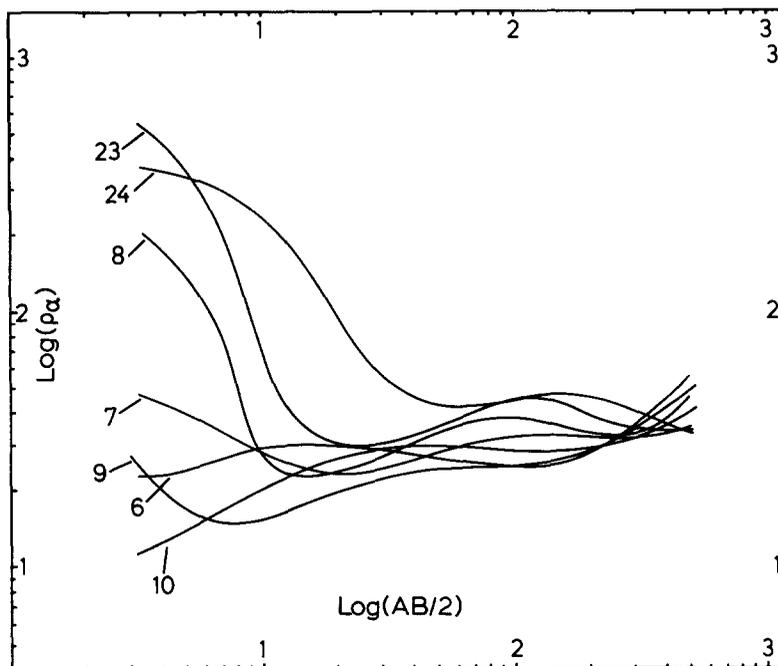
Fig. 4. Resistivity curves obtained for traverse  $T_2$ .
